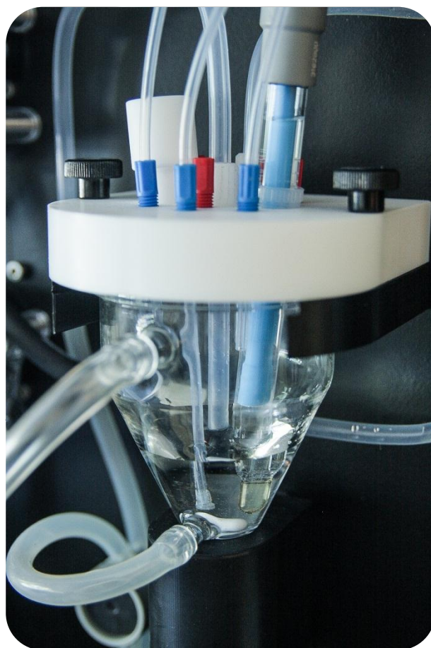
figure 5: analysis vessel with stirrer, pH probe and temp. sensor
